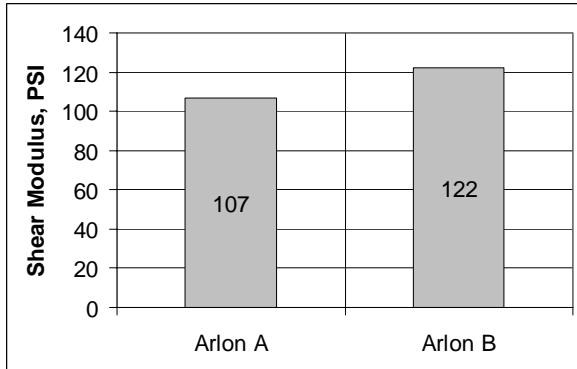
Figure 6 – Shear modulus of Arlon A and B
